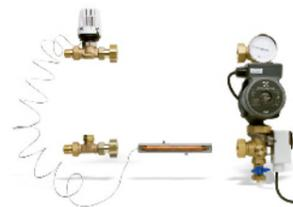
The available compact control unit may be used for the plane-sealed manifold with 1" external thread. The water inlet temperature may be set through the temperature control head. Pump and water temperature range 20-90 C, B-10kW thermal capacity; passed the pressure test.
